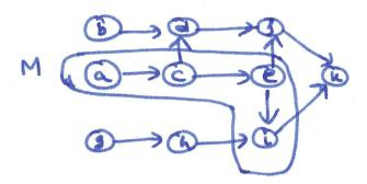
from this diagram it can be seen that the workstating that will perform tasks a and i must also preform tasks c and e. So, we can combine there Iruz tasks (a, c, e, i) into a "macro-tash" M. Obviously, the required proc. time In this new task M is tm = tattettetti= = 10 + 11 + 5 + 10 = 36 secs.
