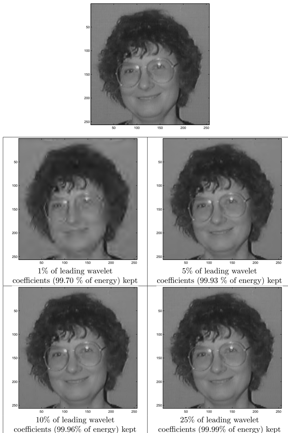
Figure 1.1: Top: true 256 \times 256 image; bottom: sparse in the wavelet basis approximations of the image. Wavelet basis is orthonormal, and a natural way to quantify near-sparsity of a signal is to look at the fraction of total energy (sum of squares of wavelet coefficients) stored in the leading coefficients; these are the “energy data” presented on the figure.
