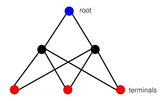
All previous algorithms solve subset k-connectivity by applying rooted k-connectivity algorithm to k terminals (pay a factor of k)
