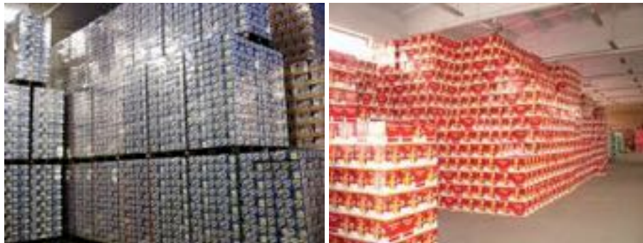
Figure 16.3: In the US warehouse on the left, cartons of beer have been palletized because labor is expensive compared to capital. The reduction in labor is worth the expense of a forklift plus the additional storage space. In the Chinese warehouse on the right, cartons have been stacked by hand and must be unstacked by hand; but labor is cheap and capital is expensive.
