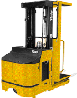
Figure 13.34. Order Picking Truck
