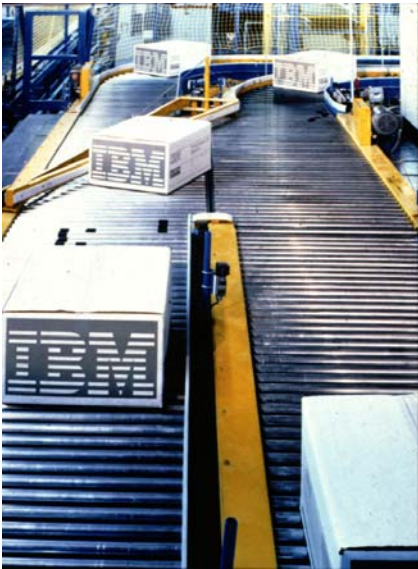
Figure 13.15. Roller Conveyor with Diverter in Electronics Manufacturing
