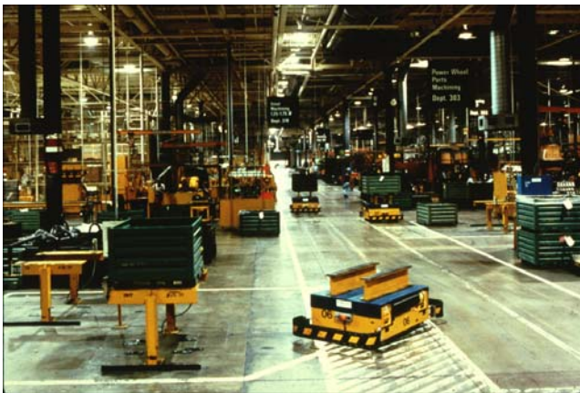
Figure 13.37. AGV with Load Station
