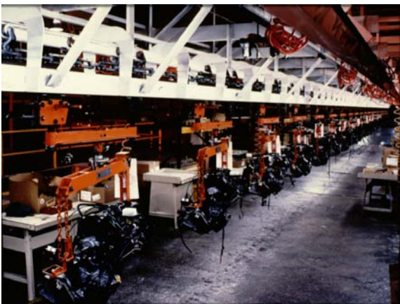
Figure 13.17. Power and Free Conveyor in Automotive Engine Assembly
