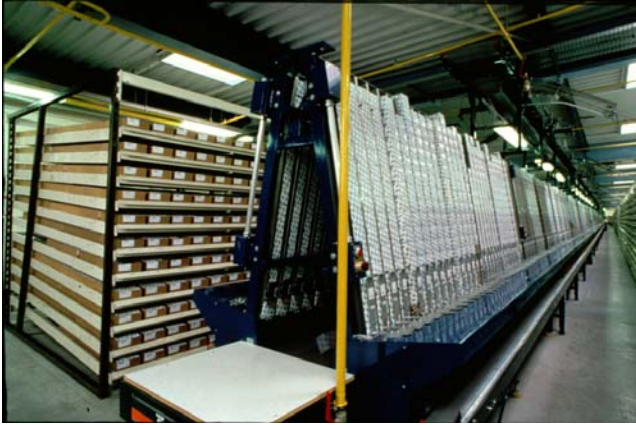
Figure 13.64. Automatic Order Picking A-Frame (Picture courtesy of Electrocom)
