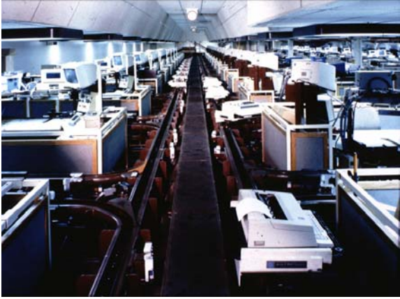
Figure 13.19. Inverted Automated Electrified Monorail in Typewriter Manufacturing
