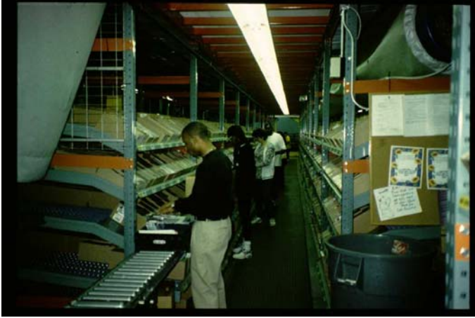
Figure 13.13. Roller Conveyor in Manual Order Picking (Photo courtesy of Dr. John Bartholdi)
