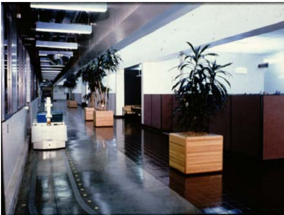
Figure 13.40. Multiload AGVS in Electronics Manufacturing
