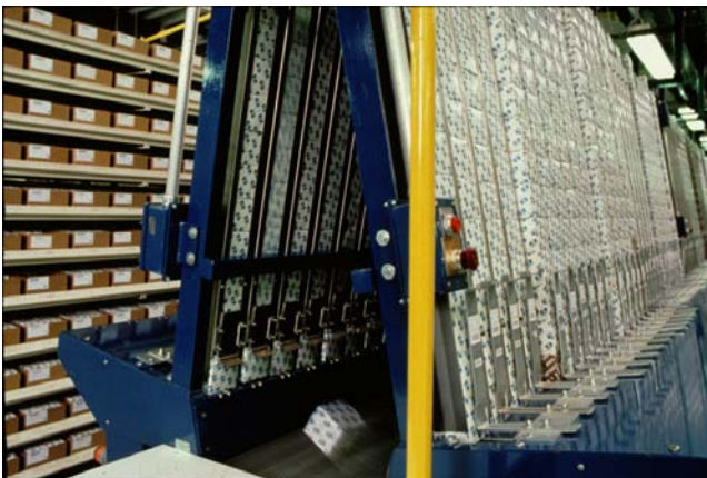
Figure 13.12. Automatic Order Picking A-Frame with Take-Away Belt Conveyor (Picture courtesy of Electrocom)
