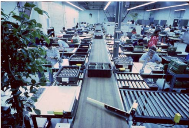
Figure 13.11. Belt Conveyor with Diverter Bar in Electronic Assembly
