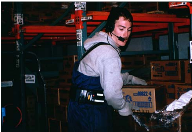
Figure 13.51. Radio-Frequency Communications during Order Picking in Cold Storage (Picture courtesy of Vocollect)
