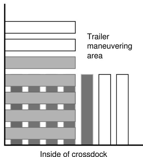
**Figure 1** An Inside Corner that Constricts Parking Space for Trailers
