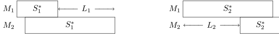
Figure 2: If S_1^* and S_2^* are processed separately, with the start times of the first jobs in each delayed without extending their makespans, then I_1^* is incurred at the beginning of S_1^* (on M_2 ), while I_2^* is incurred at the end of S_2^* (on M_1 ).
