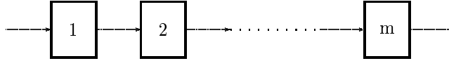
Figure 1: A simple flow line in which each item requires processing on the same sequence of work stations.
