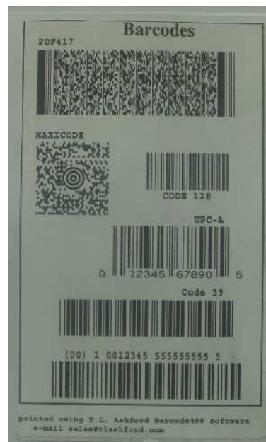
Figure 2: The top bar code is a two-dimensional stacked bar code and the next one down is a matrix bar code.
